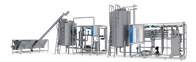
Sugar is one of the most necessary components for products such as beverages. The sugar dissolution KoomtZuc system comes ready to combine a powder dissolution system with one to dissolve sugar crystals. It is also combined with a pasteurization system making an online process of continuous dissolution with an energy-reduction process, delivering sugar syrup with °brix control.
