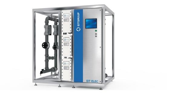
EDI systems replace the mixed resin beds to produce deionized water. Unlike the mixed resin, electrodeionization does not require continuous stops to replace or regenerate resins using chemicals. Therefore, the EDI minimizes water quality problems and operating costs.
